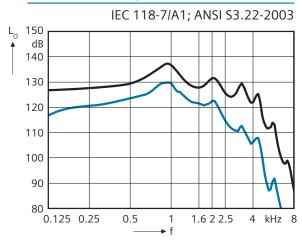
**Basic Acoustic Response** (L<sub>i</sub> = 60 dB) **Frequency Response** (L<sub>i</sub> = 60 dB)
