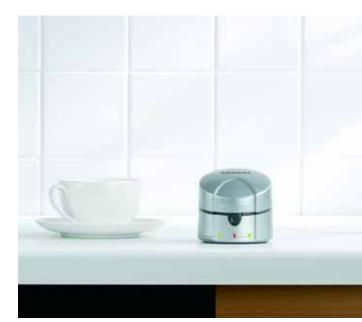
The charger selects the recharge time automatically — approximately 5 hours for a fully-drained rechargeable battery.
